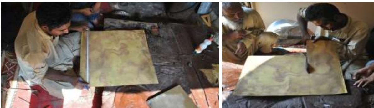
Preparing pitch and metal sheet apply on the pitch, Lahore
